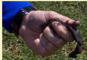
The ribbon formed here depicts a clay soil because it is greater than 1.5" in length.
