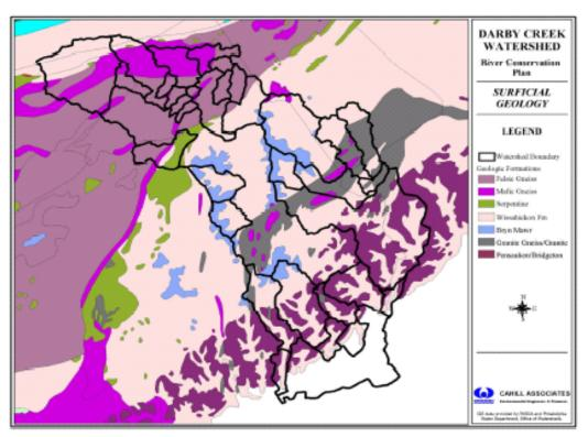
Figure III-5 USGS Geologic Composition of Darby Creek Watershed
